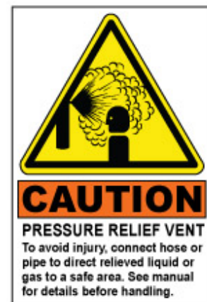
Fig. 3: Warning sticker found near the rupture disc on all meters
