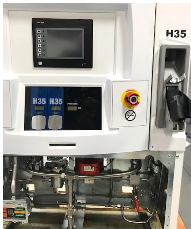
Front view of low pressure (5000 psi) hydrogen pumping station on skid.
